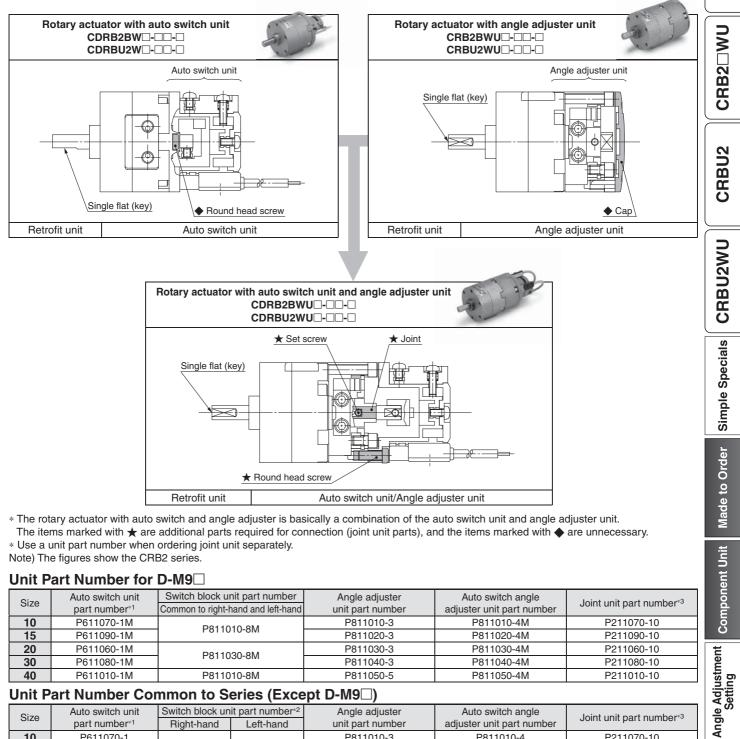
\* The rotary actuator with auto switch and angle adjuster is basically a combination of the auto switch unit and angle adjuster unit.
