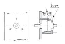
Dimension "L" of the actuators is provided in the table below for JIS standard hexagon socket head cap screws. If these types of screw are used, their heads will fit in the mounting hole.
