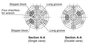
Note) For size 40, each stopper block comes with 2 holding screws.
