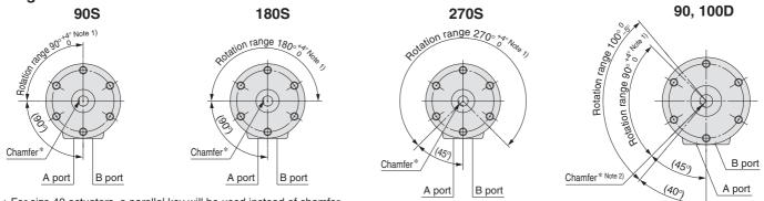
$\ast$  For size 40 actuators, a parallel key will be used instead of chamfer.
