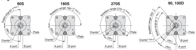
\* For size 40 actuators, a parallel key will be used instead of chamfer.
