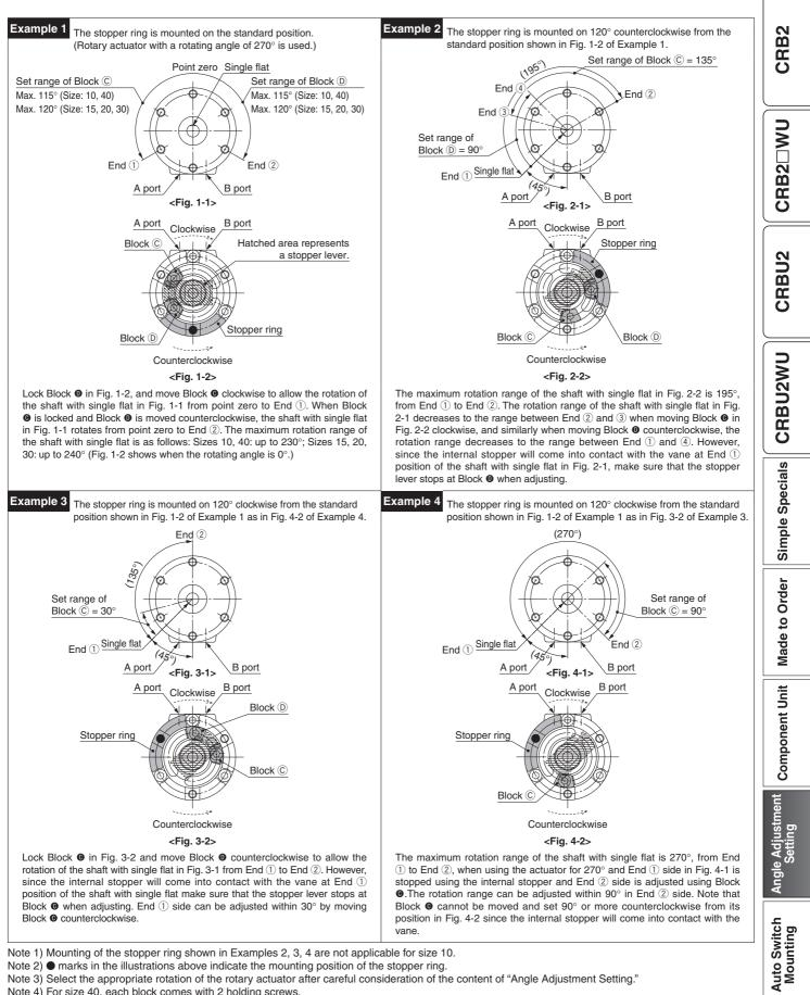
Note 1) Mounting of the stopper ring shown in Examples 2, 3, 4 are not applicable for size 10.
