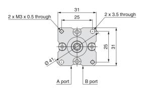
\*1. The length is 24 when any of the following are used: D-90/90A/S99(V)/T99(V)/S9P(V) The length is 30 when any of the following are used: D-97/93A The length is 25.5 when the D-M9 is used.
