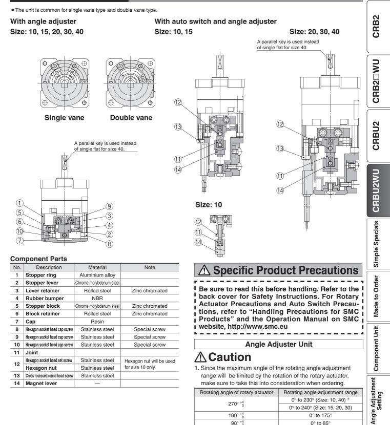
\* The maximum adjustment angle of the angle adjuster unit for size 10 and 40 is 230°.
