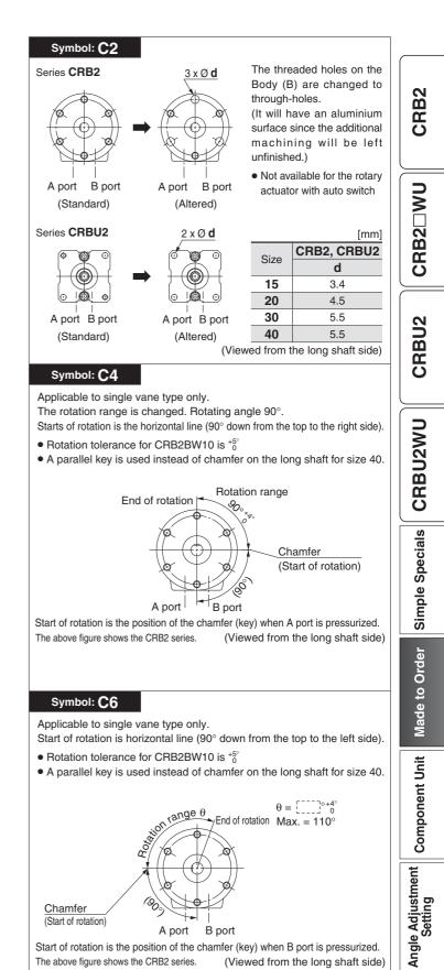
A port B port Start of rotation is the position of the chamfer (key) when B port is pressurized. The above figure shows the CRB2 series. (Viewed from the long shaft side)
