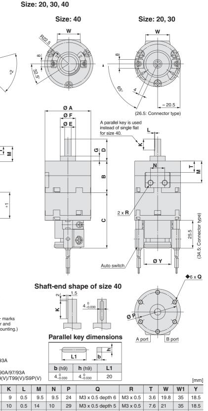
Size Α В С D **E** (g7) **F** (h9) G 4-0.004 9\_0.036 10 29 15 45.5 14 3 12\_0.043 15 34 20 47 18  $5^{-0.004}_{-0.016}$ 4 6-0.004 14\_0.043 20 42 51 20 4.5 10 36 M4 x 0.7 depth 7 M5 x 0.8 10.5 29 0.5 20 13 22 \_\_\_\_ 25 30 50 40 55.5 22 8-0.005 16\_0.043 5 12 1.0 26 14 43 M5 x 0.8 depth 10 M5 x 0.8 14 24 25 10-0.005 25\_0 0\_052 40 M5 x 0.8 depth 10 63 45 62.2 6.5 31 20 56 M5 x 0.8 17 30 30 20 31
