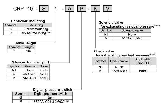
Note1) DIN rail mounting bracket is included in the package. DIN rail is not supplied.
