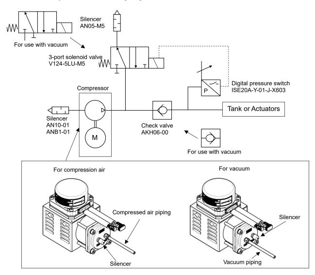
See the catalog and operation manual of the ISE20 series for piping, mounting, and details of other option parts for the digital pressure switch ISE20A-Y-01-J-X603.
