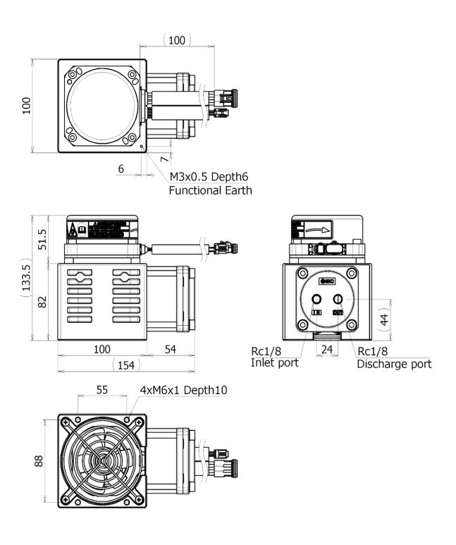
The dimensions of the controller are shown in the diagram below. 1) Screw mounting
