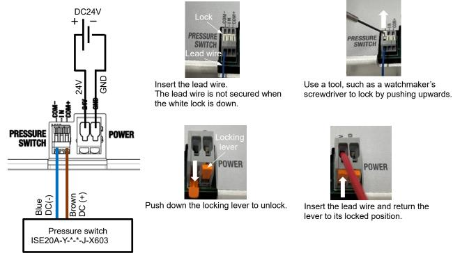
Connect the blue lead wire [DC (-)] of the pressure switch to the controller [COM-]. Connect the brown lead wire [DC (+)] of the pressure switch to the controller [COM+].
